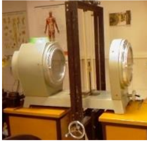
Fig. 2 Transmission polariscope (Carl Zeiss – Jena) Ø 300, white and monochromatic (sodium) light, plane and circular polarization
