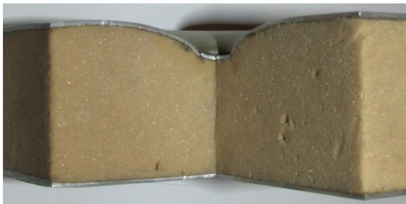
Fig. 13 An effect of the pointwise loading of the sandwich structure without reinforcement (aluminum facings, polyurethane foam core)
